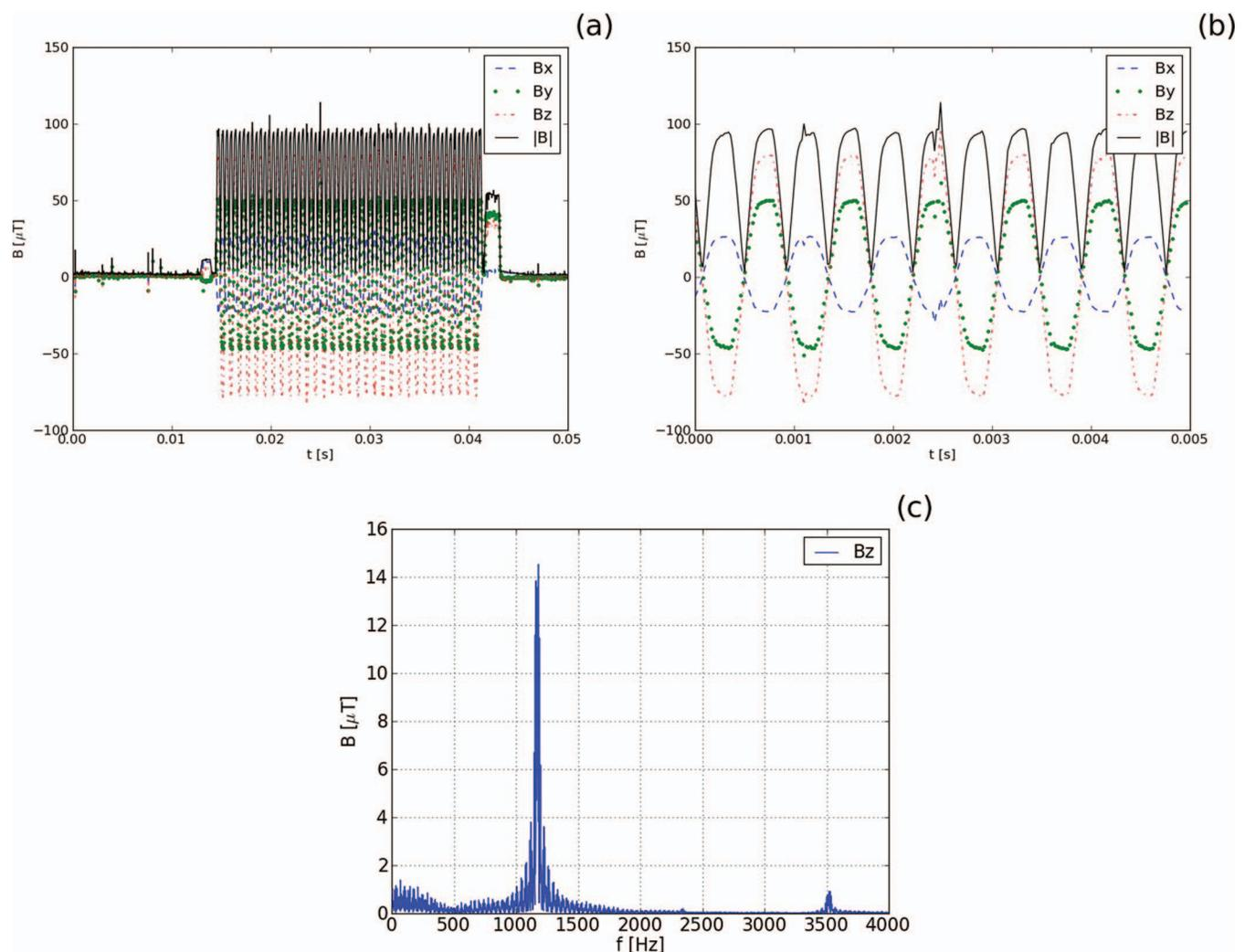
FIG. 1. GMF measurements, set H1S1: (a) in time domain; (b) in time domain with faster time base; (c) frequency spectrum (Z component).
