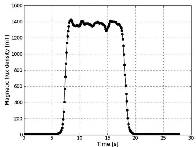
FIG. 6. SMF measurements, action A3: perceived magnetic flux density as a function of time. Description of the movement: The volunteer (miming an anesthesiologist) entered the magnet room, moved behind the gantry passing on its left, performed various movements at the rear opening of the bore (backed off, bend her torso several times, put her head inside the bore), then exited the magnet room.
