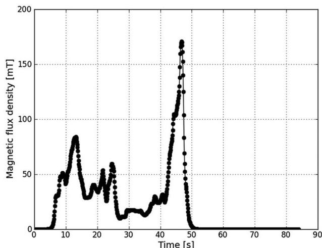
FIG. 7. SMF measurements, action A8: perceived magnetic flux density as a function of time. Description of the movement: The volunteer (miming a technician) left the control room, entered the magnet room, reached the stretcher, performed various preparations on the patient and placed the RF coil on him, raised the stretcher, and pushed it into the bore, checked the patient, then left the magnet room and returned in the control room.
