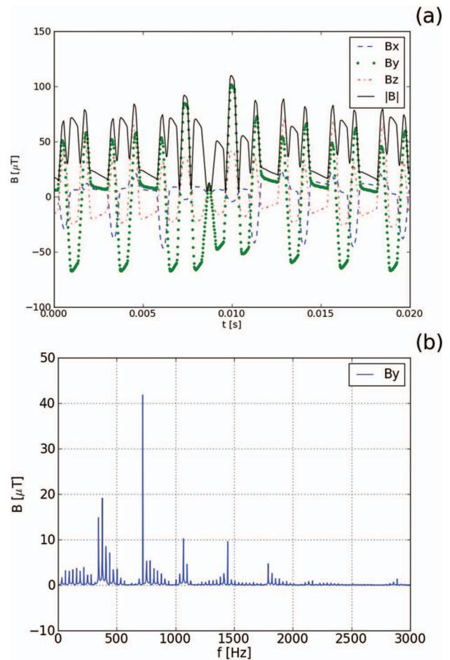
FIG. 3. GMF measurements, set H3S2: (a) in time domain; (b) frequency spectrum (Y component).
