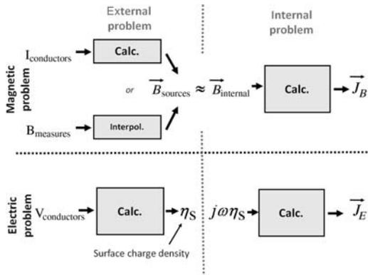
Figure 3. Sub-problems in calculation of low-frequency current density by means of quasi-static methods.
