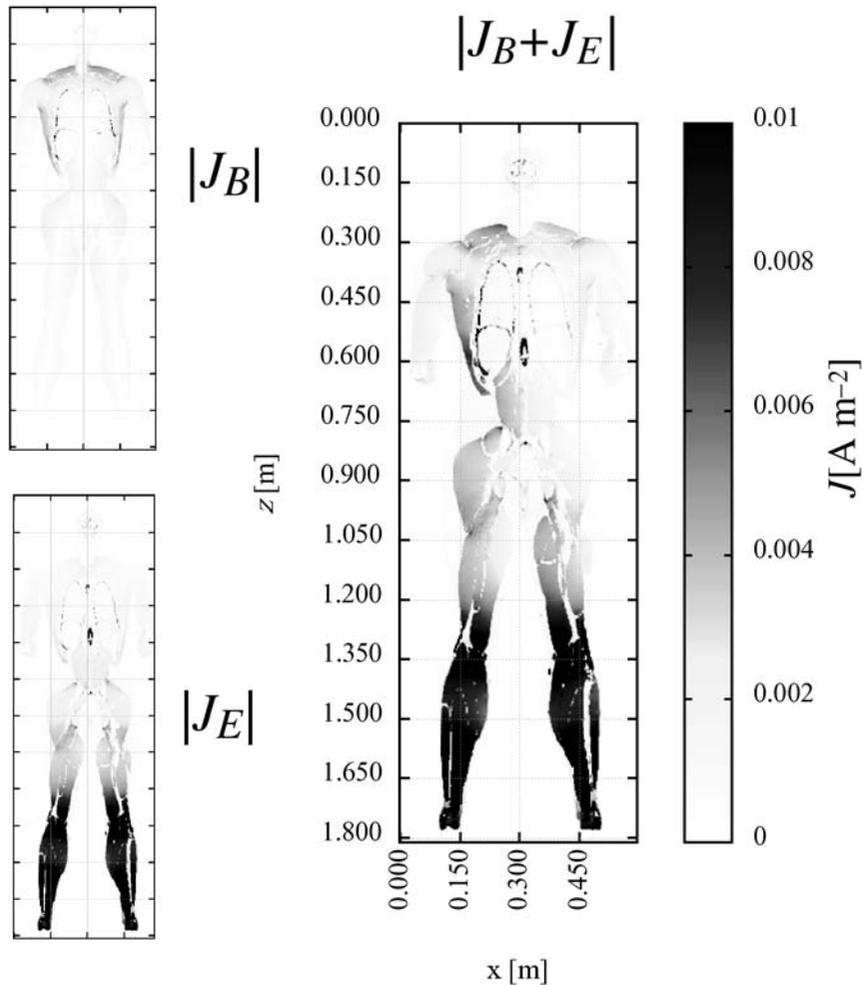
Figure 4. Composition of ‘magnetically’ and ‘electrically’ induced current densities on a sagittal section of the exposed subject.
