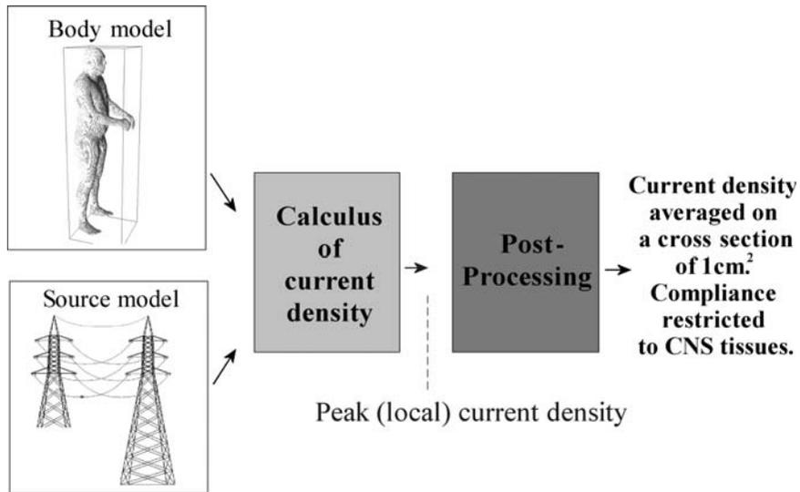
Figure 1. Main elements in a numerical study of the current density induced in the human body at low frequency.
