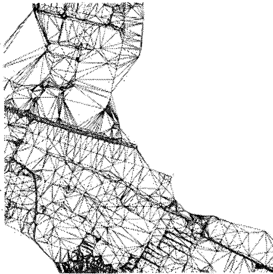
Fig. 6 - Digital three-dimensional model of the terrain (DTM) of the zone within the dotted rectangle of Fig. 5.
