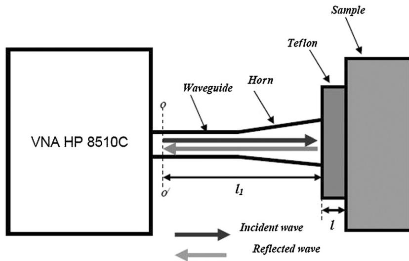
**Figure 9.** Schematic representation of the VNA matched to the waveguide with the horn antenna terminated by a Teflon plate with the sample under investigation. Here  $l_1$  is the distance from the section  $OO'$  to the Teflon plate and  $l$  is the thickness of the Teflon plate.
