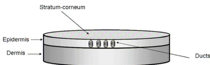
**Figure 5.** The model used for 3D electromagnetic simulations. The disk represents a portion of skin consisting of three separate layers and an array of eight sweat ducts. (Reproduced with permission from Feldman *et al* (2008); Copyright 2008, American Physical Society.)
