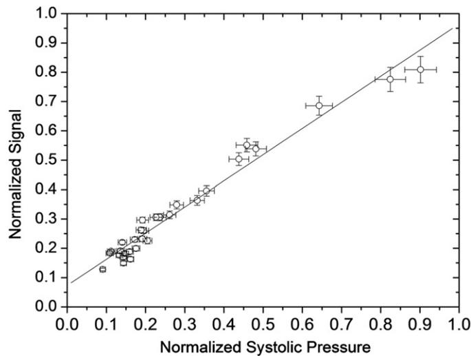
**Figure 14.** The correlation graph between the systolic blood pressure and  $\langle W_{\text{rel}}(t) \rangle_f$ , obtained from the average of 13 subjects measured as they relaxed for a period of 30 min after intensive physical activity (Feldman *et al* 2008). (Reproduced with permission from Feldman *et al* (2008); Copyright 2008, American Physical Society.)
