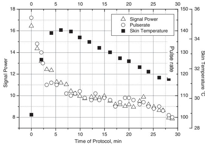
**Figure 12.** The typical time behaviours of the signal power obtained from the reflection coefficient of the subject’s palm, a concurrent pulse of the same person at rest following intense exercise and the temperature of the subject’s skin. The subject is a Caucasian male aged 35.
