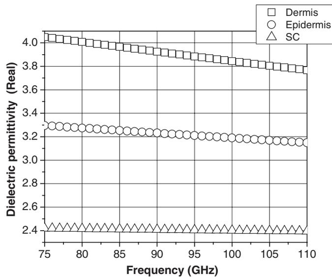
**Figure 3.** The dielectric permittivity of different skin layers in the frequency range from 75 GHz to 110 GHz. For clarity, only the real component of the dielectric permittivity is shown.
