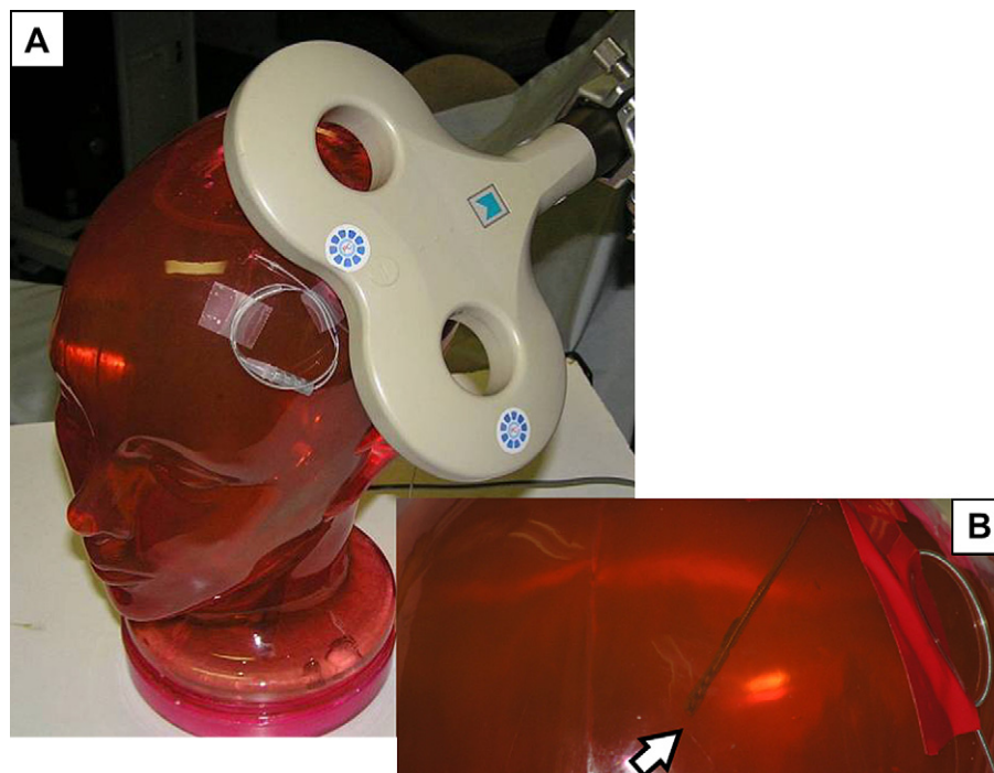
Fig. 1. Head phantom and insulated DBS lead for TMS. The head phantom was filled with gelatin, which was adjusted in thickness and impedance to be similar to those of human brain. The DBS lead was inserted into the phantom through a hole in the left frontal position (A). The tip of lead was positioned at the hypothetical subthalamic nucleus (B). The extra lead was fixed with or without double loops near the insertion point.
