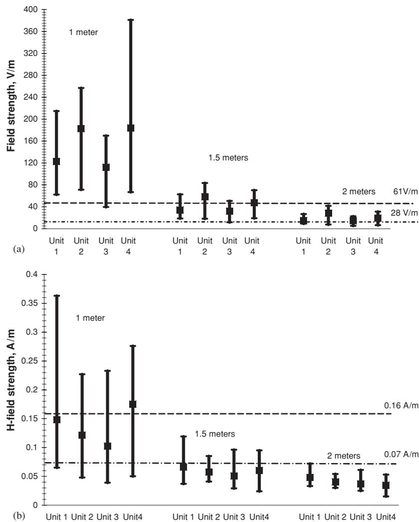
**Figure 3.** (a) The maximum, minimum and mean  $E$ -fields emitted by four capacitive CSWD units with medium-sized electrodes relative to the distance from the unit. (b) The maximum, minimum and mean  $H$ -fields emitted by four capacitive CSWD units with medium-sized electrodes relative to distance from the unit.
