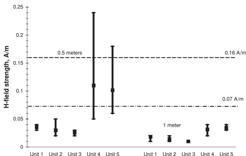
**Figure 7.** A comparison of the range of  $H$ -field values recorded for all inductive PSWD units at 0.5 m and 1.0 m from the unit.
