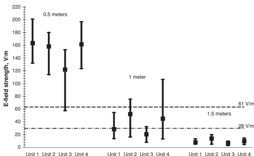
**Figure 5.** *E*-fields emitted by capacitive PSWD with medium-sized electrodes relative to distance from the unit.
