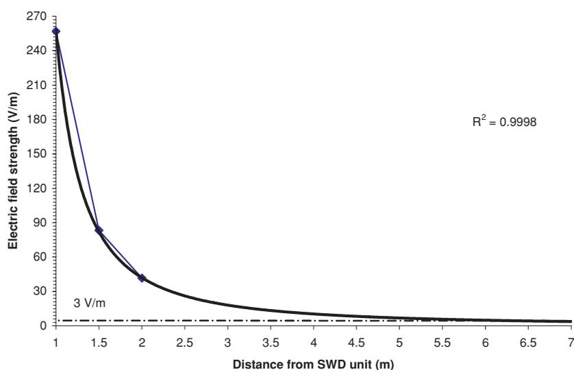
**Figure 8.** Predicted trend in stray fields emitted compared with electromagnetic compatibility levels.
