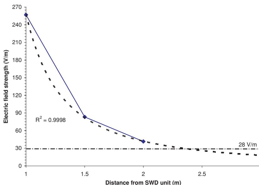
**Figure 9.** Predicted trend in electric field strength levels for capacitive CSWD.
