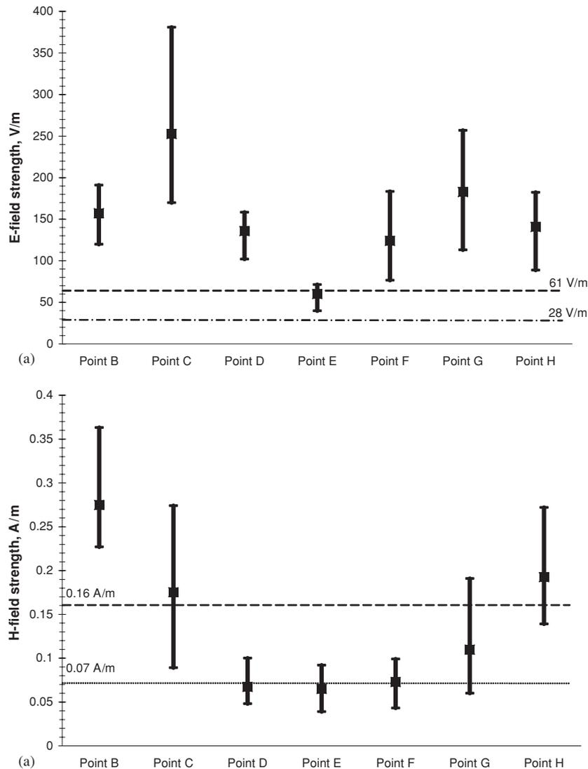
**Figure 4.** (a) The maximum, minimum and mean  $E$ -fields levels at points B–H, 1 m from capacitive CSWD units with medium-sized electrodes (measurements at point A were not taken due to the length of the units). (b) The maximum, minimum and mean  $H$ -field levels at points B–H, 1 m from capacitive CSWD units with medium-sized electrodes (measurements at point A were not taken due to the length of the units).
