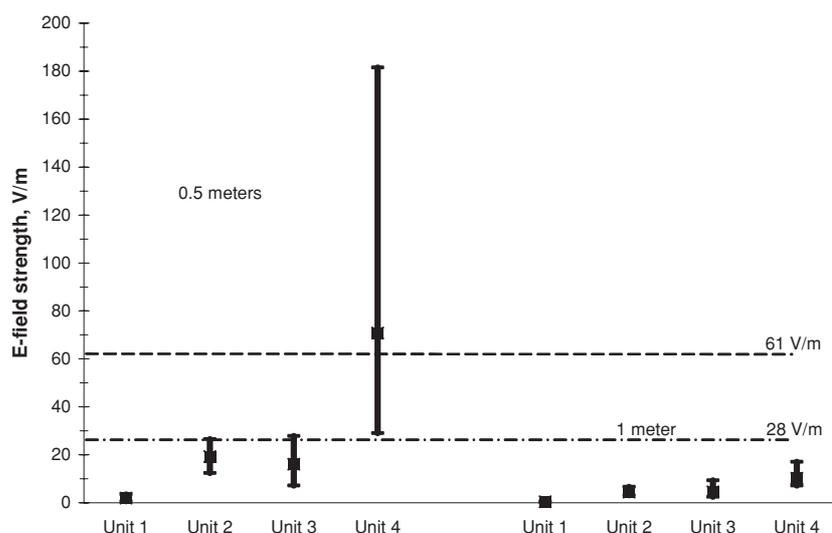
Figure 6. *E*-fields emitted by inductive CSWD at 0.5 and 1 m from the unit.
