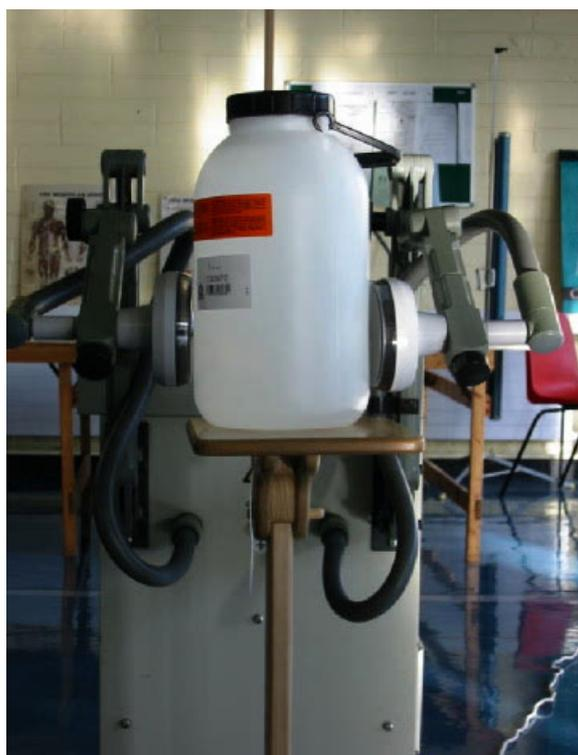
**Figure 2.** Phantom electrode configuration for testing the capacitive method (for the inductive method, the electrode was positioned at one side of the phantom).
