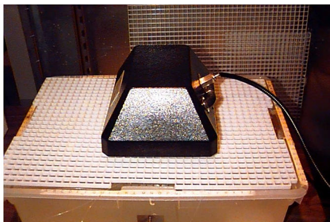
Figure 2. Diathermy applicator on support grid of the exposure phantom box.
