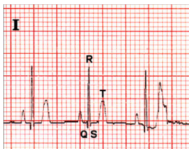
Figure 3. Lead I electrocardiographic tracing generated by a patient signal simulator. Three consecutive QRS complexes are shown: the last one after having positioned the hand-held electrode in close proximity to the ECG device. EMI caused the elevation of the ST segment and depression of the R wave.
