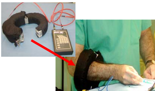
Fig. 5. The clamp-on meter for measurements of the current in the surgeon's hand
