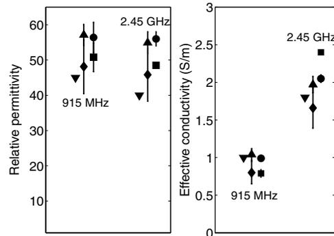
**Figure 2.** Comparison of the relative permittivity and effective conductivity (S/m) of *ex vivo* data in this study (normal (◆), malignant (▲)), with data reported in Stauffer *et al* (2003) (normal (■), malignant (●)), and Gabriel *et al* (1996a) (normal (▼)). The error bars for this study correspond to the standard deviation. The error bars for the Stauffer *et al* (2003) study correspond to the range of data given. No range is provided in Gabriel *et al* (1996a).
