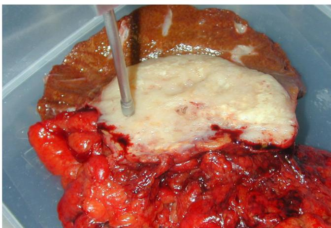
**Figure 1.** Dielectric spectroscopy of an excised liver tumor (light-colored mass), using a precision open-ended coaxial probe (shown with the tip making contact with the tissue).
