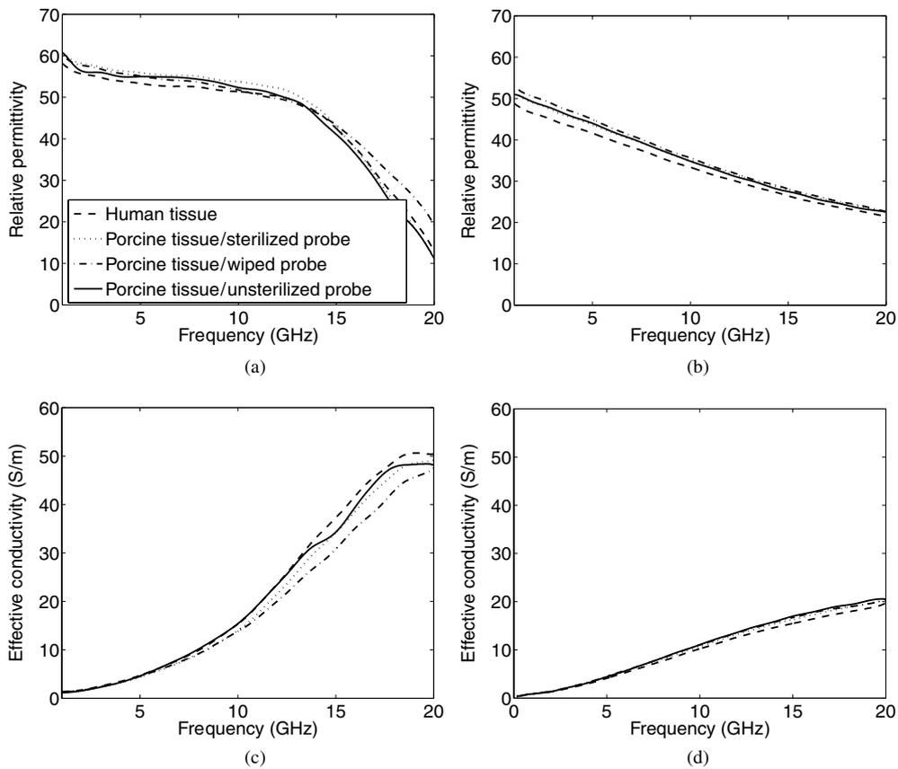
**Figure 5.** Comparisons of dielectric properties data for normal human liver tissue and various probe measurement scenarios with porcine liver. (a) *In vivo* relative permittivity, (b) *ex vivo* relative permittivity, (c) *in vivo* effective conductivity and (d) *ex vivo* effective conductivity.
