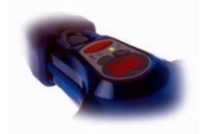
This remote operation offers the ability to configure Magstim stimulation equipment through the stimulating coil and is achieved by integrating pulse strength selection ( $\blacktriangle \nabla$ ), parameter display, trigger and stop buttons into the coil handgrip to facilitate total system control via the coil.
