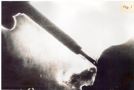
Fig. 1: Schlieren Photography during electrotomy.
